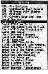
To change the Data Fields, press MENU from the Moving Map and select SETUP DATA FIELDS. You will be brought back to the Moving Map where one of the Data Field boxes will be highlighted in light blue. Move the highlight to the desired Data Field box to change and press ENTER to bring up the list of available Data Fields (see above). Select the new Data Field and press ENTER to set it.
