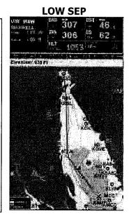
Once TAWS is active with a position fix, there will be a small box in the lower left hand corner of the Moving Map:
