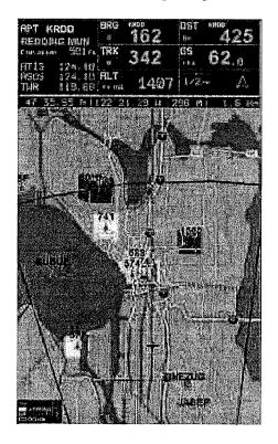
The AUTO setting for TAWS allows the EKP-IV to calculate the appropriate setting for you, based on the OCH. Once the OCH reaches 3,000 feet, the EKP-IV will switch to HIGH SEP, and in areas below an OCH of 3,000 feet the EKP-IV will operate in LOW SEP.
