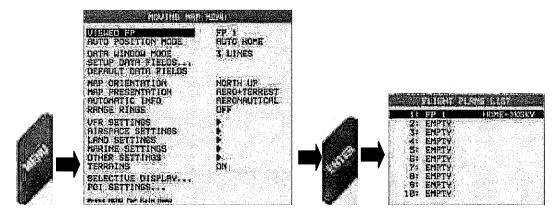
If the current Flight Plan is active, then a warning will be displayed that the Flight Plan will be deactivated prior to switching the Viewed FP.
