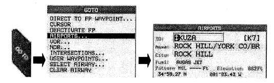
If an airport is used for the direct waypoint, then once it is selected, the toggle can be used to scroll through the Frequencies, Approaches and Runway info on that specific airport.
